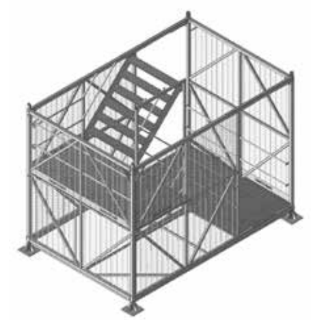
Step 10: Top Stair Flight Installation
